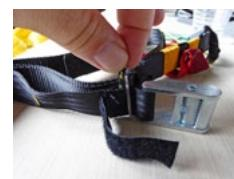
Extract the webbing system, complete with Kamet buckle (photo) and replace with the new replacement part in the reverse order. Be sure to replace the magnet with the correct polarity, securely into the inner pocket flap so as it cannot fall out.
