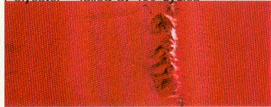
Polyester – failed at 459 cycles
