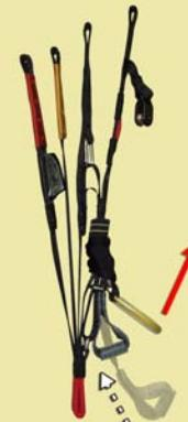
**Trimmers released (C & D straps of the risers are longer than A & B)**
