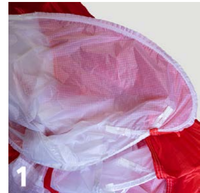
Turn the leading edge inside out. Photo 1
