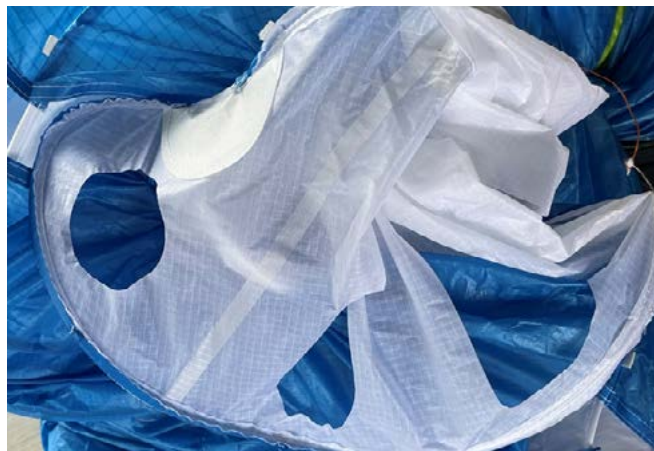
Turn the leading edge inside out. Photo 1
