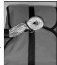
*The elastic ring used to close the container is threaded through the eyelets on the container flaps to draw it closed.*
